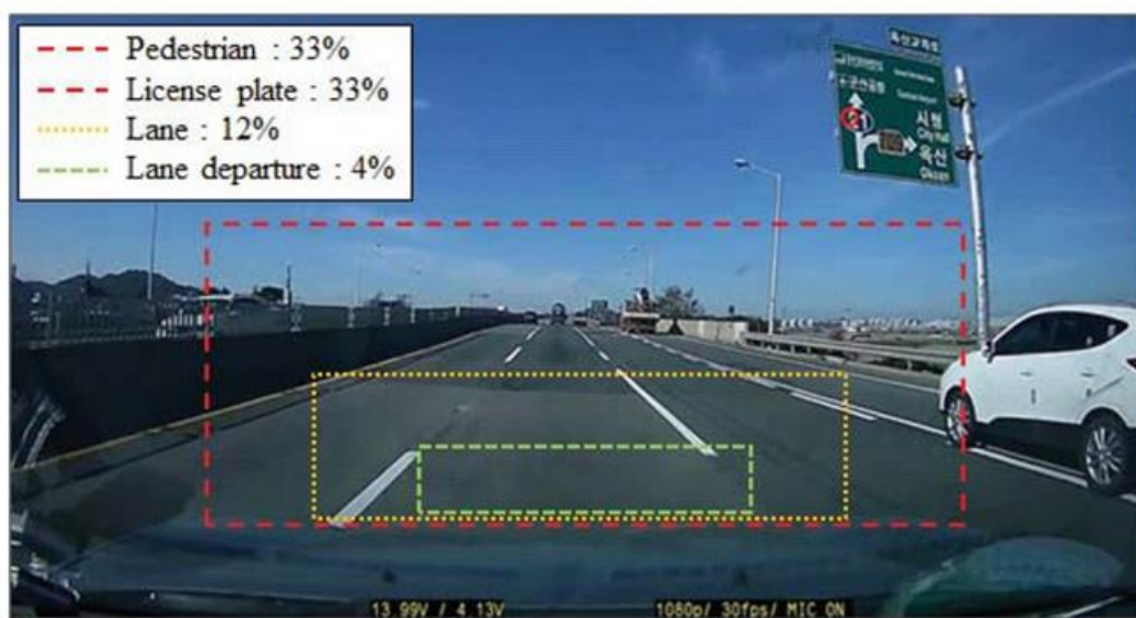
Size of static ROI to recognize objects on the road
